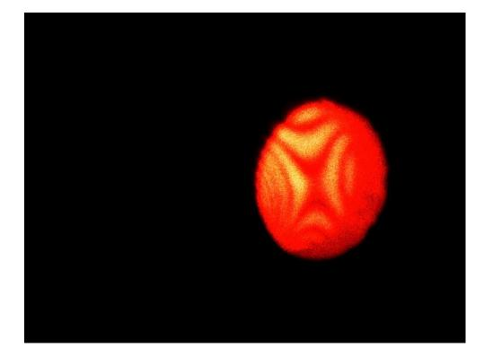
When a sound is played near the interferometer, the pellicle beam splitter vibrates, changing the fringe patterns.
