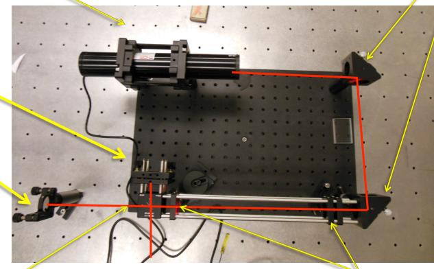
Pellicle Beam Splitter Positive Lenses- 2 create a telescope to expand the beam
